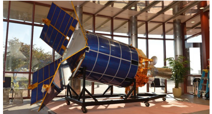
The one-half scale model of a Defense Support Program (DSP) satellite used for space-based missile warning is preserved at Buckley Air Force Base.
