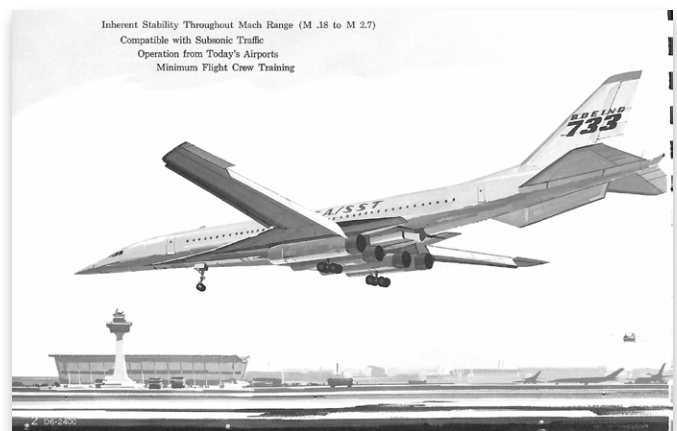
Artist’s depiction of the landing configuration of the Boeing Model 733 Supersonic Transport as depicted in Boeing’s Commercial Supersonic Transport Proposal of January 15, 1964.
