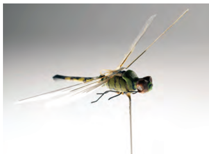
Developed by CIA's Office of Research and Development in the 1970s, this micro unmanned aerial vehicle (UAV) was the first flight of an insect-sized vehicle (insectohtoper) intended to prove the concept of such miniaturized platforms for intelligence collection. It had a miniature engine to move the wings up and down. A small amount of gas was used to drive the engine, and the excess was vented out the rear for extra thrust. The flight tests were impressive. However, control in any kind of crosswind proved too difficult.
